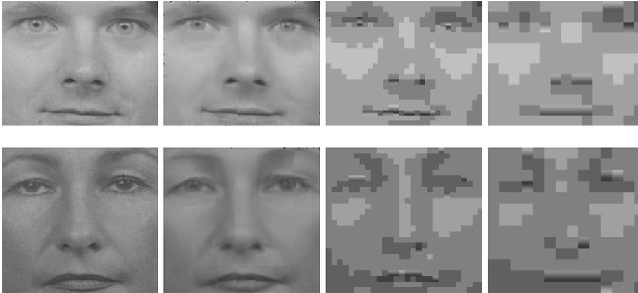
Figure 3.5: *First column: original images (not included in training set). Second column: block-tiling with block size  $[32 \times 32]$  pixels, PSNR = 33.6 dB and 33.3 dB (top and bottom, respectively), rate = 0.07 bpp. Third column: JPEG encoded, PSNR = 27.0 dB and 26.6 dB, respectively, rate = 0.18 bpp. Fourth column: subsampled JPEG: PSNR = 25.4 dB and 25.3 dB, rate = 0.12 bpp*
